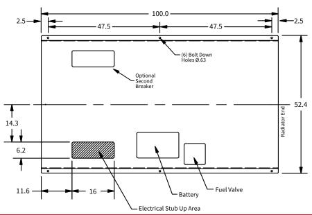
Note: The above drawings are provided for reference only and should not be used for planning installation.
