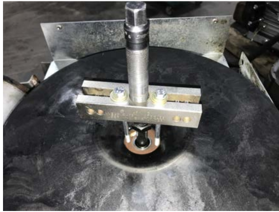
FIGURE 64. PULLING FAN HUB OFF ROTOR
