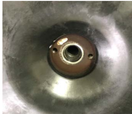
FIGURE 62. FAN HUB AND END OF ROTOR
