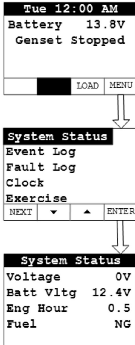
FIGURE 31. SYSTEM STATUS SCREEN
