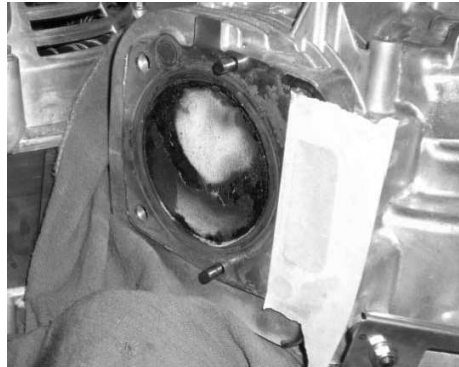
FIGURE 7. PUSH ROD PORTS WITH MASKING TAPE
