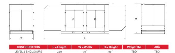
\* All measurements are approximate and for estimation purposes only. Weights are without fuel tank. Sound levels measured at 23ft (7m) and does not account for ambient site conditions.
